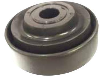
CDM Mountings are used in pairs, providing a simple single bolt installation. They are able to withstand high dynamic shock loads, particularly when being used on Off-Road Vehicles. The outer body incorporates a steel cup to limit vertical movement and reduce rubber stress, normally caused by bump & shock conditions.
