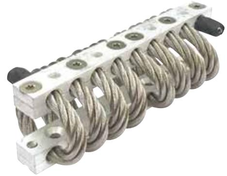
Wire Rope Shock mountings are an "All Metal" design, providing multidirectional absorption of High Level Shock and Vibration. The all-metallic design allows these mountings to be used in extremely harsh conditions, including corrosive and high temperature environments.
