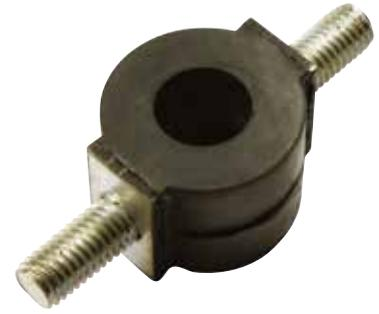
High performance mountings for lightweight equipment. They are designed to give high levels of deflection under light loads, providing a low natural frequency and high levels of vibration isolation – both Active & Passive. They can be used in either compression, shear or a combination.
