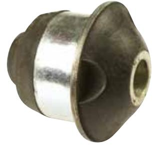
Utilising the rubber primarily in shear, Flanged Bushes have a high radial to axial stiffness ratio and are therefore ideal for controlling horizontal movement. They are a relatively stiff mounting, suitable for carrying loads of up to 1100Kg per mounting and are ideal for high frequency vibrations. Using top and bottom washers provides a fail-safe installation.
