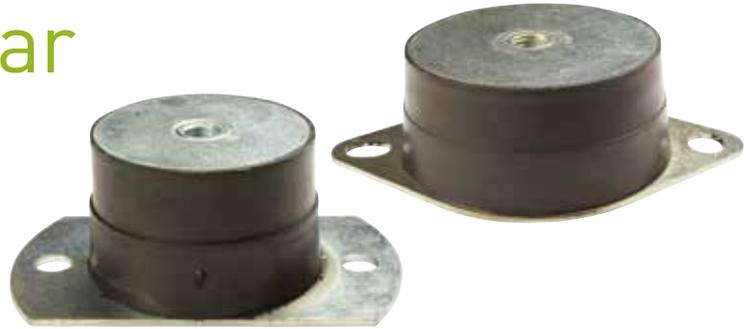
Flanged Circular Mountings are a simple, low cost, compression mounting and provide good levels of vibration reduction. The mountings are produced with or without a metal interleaf. The interleaf provides increased load capacity.
