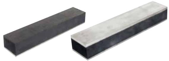
Heavy Duty and Robust - Rail Mountings are ideal for supporting heavy plant and machinery. They can be supplied in up to 2 meters in length, with top and bottom metals, or bottom metal only. Suitable for use in Compression, Shear, or a combination of both.
