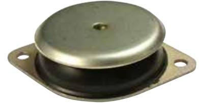
Flanged Mountings give high levels of deflection, providing excellent levels of vibration reduction and shock absorption both in the vertical and horizontal planes. They are particularly suited to isolating slow speed equipment.
