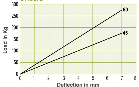
Max compression load in Kg deflection in mm.
