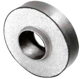
Armoured Plate Mountings are used to allow flexibility within an installation and reduce stress on brackets and fabrications. They are typically used in pairs, on opposing sides of a bracket, to allow for vibration isolation in the positive and negative direction.
