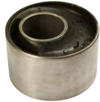
Eccentric Bushes are manufactured from two metal sleeves which are eccentrically offset in the radial direction. This offset allows for a larger proportion of the rubber section to be orientated in the normal direction of load, allowing for relatively large radial deflections to be achieved, whilst maintaining excellent motional control characteristics.
