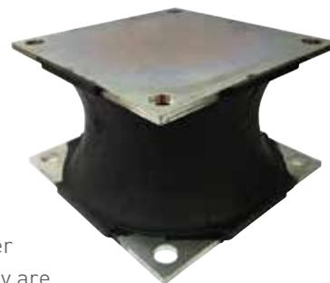
Shear Compression Mountings are manufactured from high quality natural rubber and are designed to allow large amounts of horizontal and lateral movement. They are typically used in the Construction Industry, particularly on Compaction Equipment. The high grade rubber formulation ensures extended service life under continuous high levels of mechanically induced vibration.
