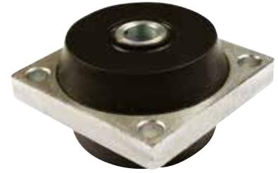
Multi Directional mountings are used to accommodate forces in both the upwards & downwards direction (i.e. positive and negative forces), and are ideal for applications such as Gearbox mountings where the torque applied during forward and reverse situations needs to be accommodated. Mountings should be used with Top & Bottom overload washers to provide a failsafe mounting arrangement.
