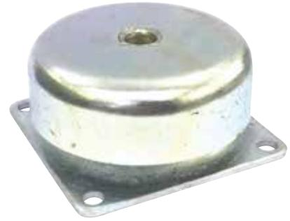
Cup Shock mountings are a relatively stiff product, ideal for applications where high frequency vibrations are predominant. The product is failsafe and ideal for both mobile and static applications. The outer metal cap offers protection from contaminants such as Oil and Fuel. The design of the mounting also allows the product to be used in tension, although maximum loads should be derated.
