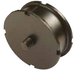
Bemag mountings are used primarily within the Construction Industry and can accommodate high dynamic forces. The oversized end metals allows for improved bonded interface between the rubber and metal to increase the fatigue life, particularly where continuous dynamic forces are applied in shear. Available with M12 threads on request.
