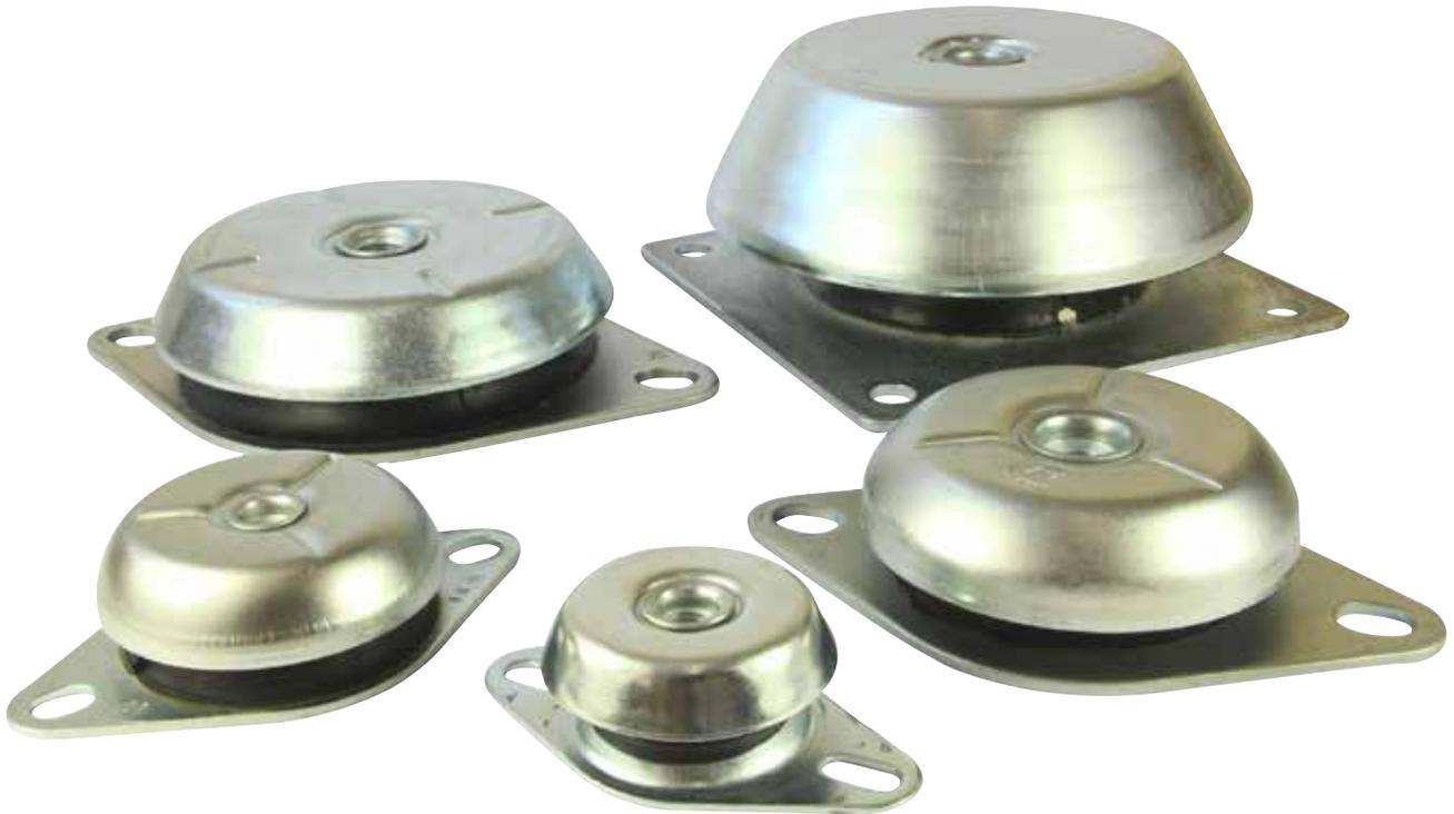
A universal mounting, popular in a wide range of applications. Cost Effective, High Performing and Easy to Install. The rubber is used in shear compression providing optimum performance and offers vibration reduction of up to 95% in all axis. The metal top cap provides protection from contamination such as Oil and Fuel. Load Ratings from 20kg to 5,000kg.
