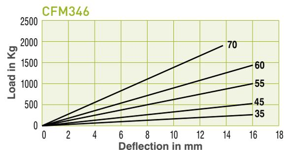
Max compression load in Kg deflection in mm.
