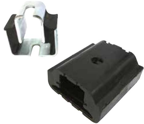
UU Shear mountings are designed to load the rubber in shear and thereby provide a soft vertical spring rate and high levels of vibration absorption.
