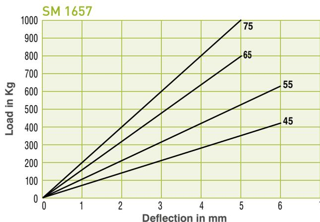
Maximum Loads should be derated for marine propulsion engines.
